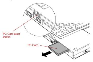
Figure 3-2 Removing the PC Card
